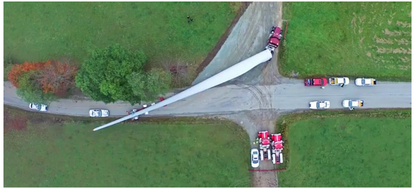
A drone captures a blade trailer negotiating a turn. This highlights the “tip swing” and difficulty turning on the typical rural roads near the final project site. (Courtesy: Logisticus Project Group, LLC)
